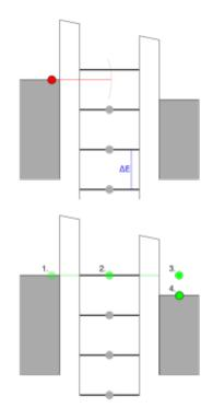
The energy levels of the island electrode are evenly spaced with a separation of \$\Delta E\$. This gives rise to a self-capacitance C of the island, defined as
